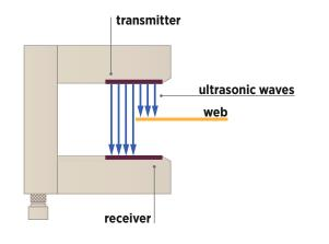
SU.m-25 is equipped with two ultrasonic capsules, the transmitter one generates an ultrasonic wave sequence every 3,5 msec which is converted into electric signal by the receiver one. According to the intensity of the signal received, the microprocessor can identify how much of the sensitive surface of the capsule is covered by the material inserted in the fork and calculate the position of the web edge.
